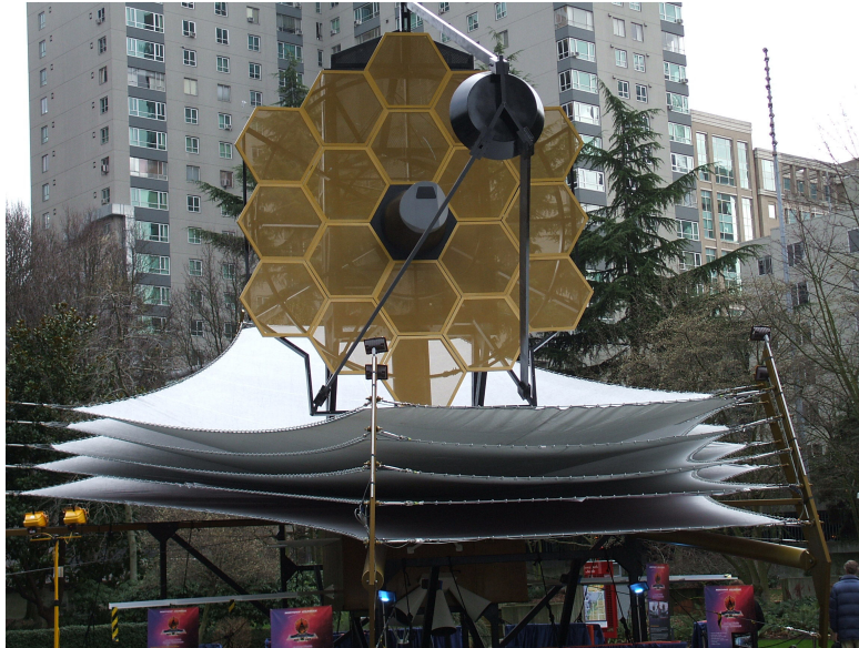
Figure 21: A mock-up of the James Webb telescope, displaying its five-layered sunshield.
